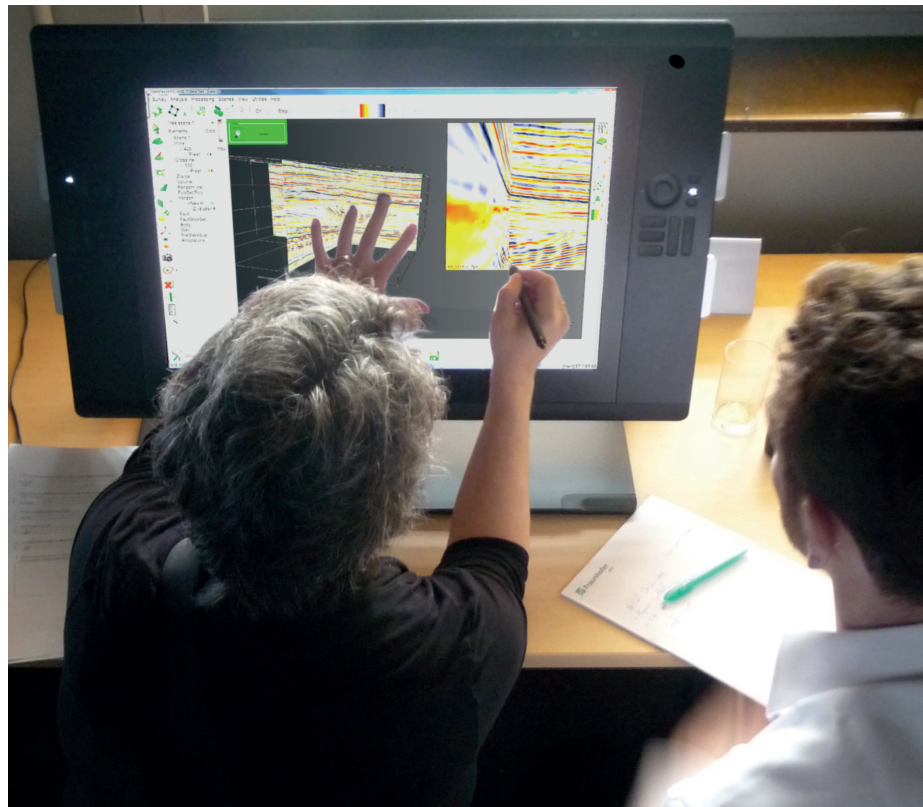
Figure 7.1: Single user during the picking of seeds using the lens-mode [ @VRG ]
