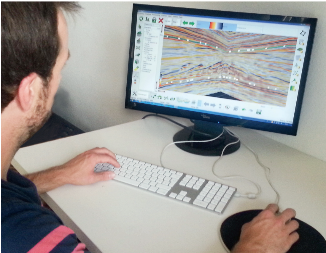
Figure 4.11: Seed picking in OpendTect using traditional input devices. While seeds are picked on the Graphics Window, mode switches are executed on the Command Window
