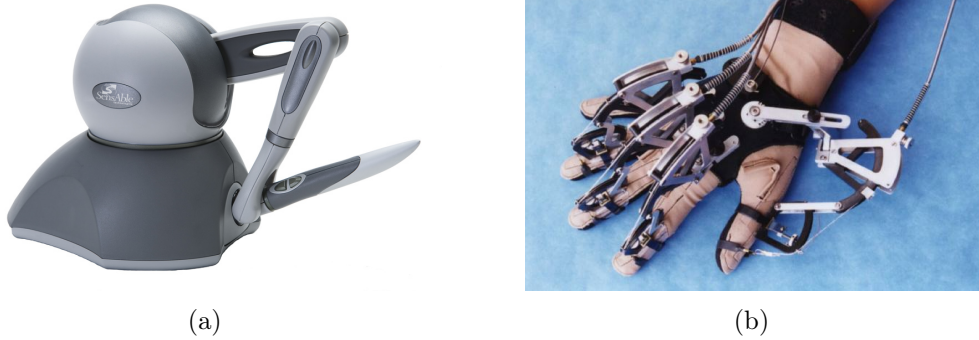
Figure 3.5: Two haptic displays. (a) A version of the ground-referenced Phantom with an integrated stylus-like device. (Image courtesy of SensAble Technologies, www.sensable.com ) (b) The CyberGrasp haptic force display. (Image courtesy of Immersion Corporation, www.immersion.com )
