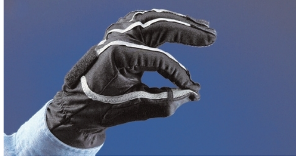
Figure 3.6: The Pinch glove, a discrete VR input device. (Image courtesy of Mechdyne former Fakespace Corporation, www.mechdyne.com )
