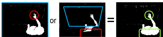
Figure 2: A combination of depth segmentation (left image) and IR-intensity segmentation (middle image) leads to better segmentation results (right image) and solves the respective problems (see regions in green circles). The red circles indicate the problematic regions in depth-based segmentation (left) and IR-based segmentation (middle), respectively.
