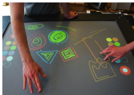
Figure 6: User awareness allows assigning individual tools to each touch event. Here, each user draws with an individually selected color.
