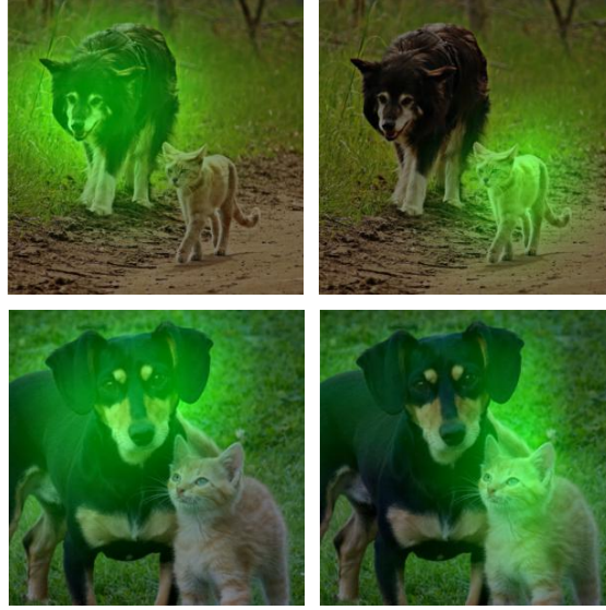
Figure 39: Comparison of Grad-CAM heatmaps for classes cat (right) and dog (left) on Inception V3
